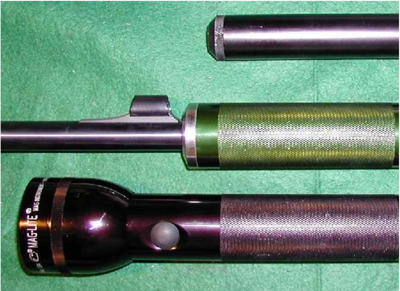
The silencer can be dismantled through the original opening where the batteries would normally go. The end where the silencer screws onto the rifle is permanently closed with a stainless steel bushing that I pressed inside the flashlight, I made the bushing so it was a slightly bigger in diameter and would just get stuck inside the flashlight tube. I also made an area with a smaller diameter on the bushing where I put on some binary epoxy-gluue to ensure it staying there.
