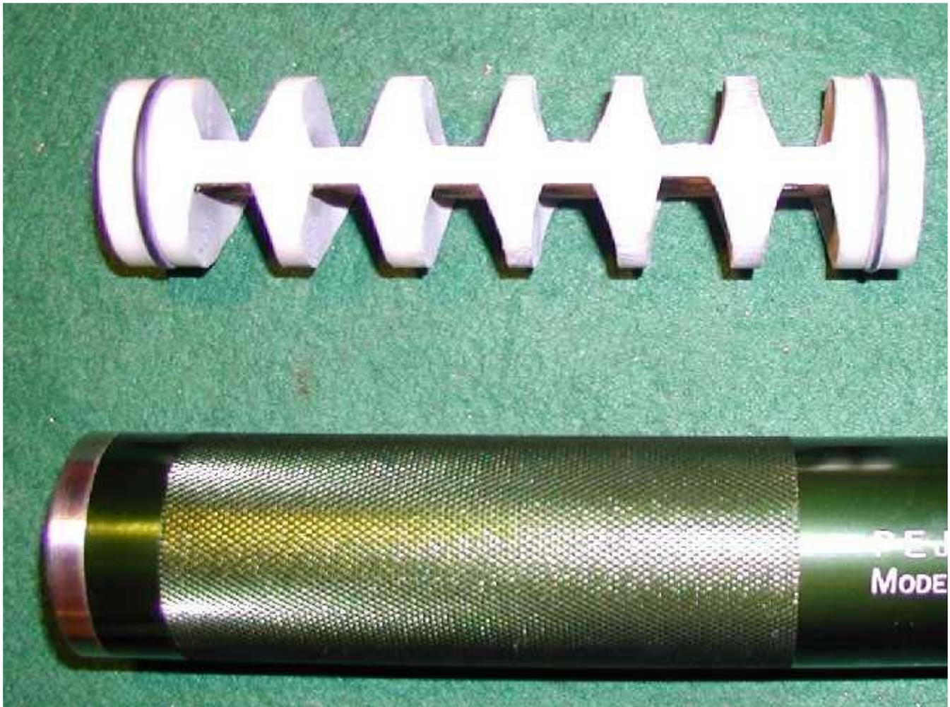
In this picture, you can see the delrin-rod have been turned about 90 degrees. You can see the rod has a hole for the projectile all the way through and that there's much room for the gasses to escape into the 6 smaller spaces. In principle it's just like taking washers and springs - this is just one part with everything
